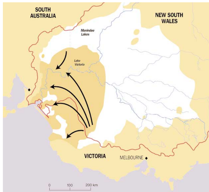
Figure 5: The extent of the Murray Group aquifer in the Murray Basin. The arrows show the direction of groundwater flow in the aquifer. Source: Evans et al. 1990.
